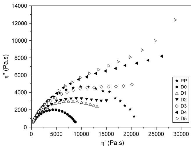
Fig. 8. Cole–Cole plot of the plain PP and modified PPs at 180 °C.
