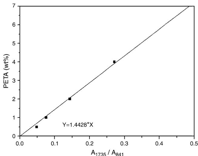
Fig. 3. Calibration curve for the determination of the percentage of reacted PETA in PP-g-PETA.
