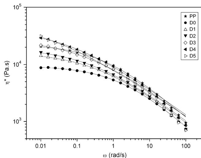
Fig. 4. Complex viscosity vs. angle frequency for the plain PP and modified PPs at 180 °C.
