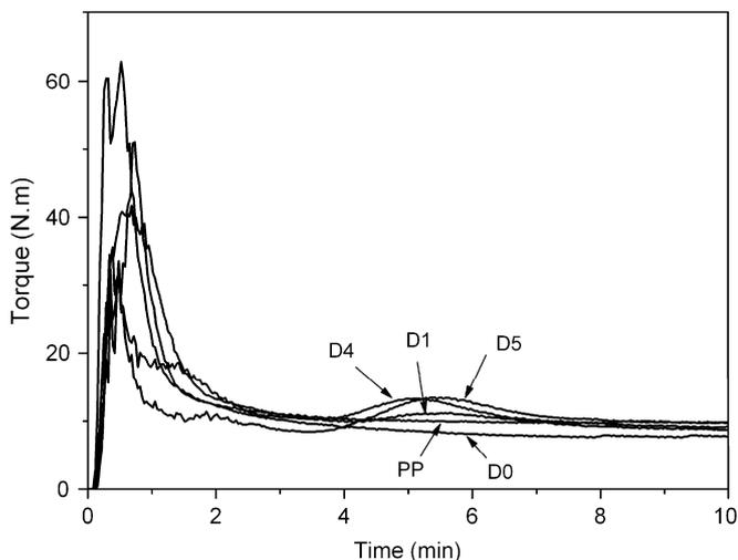
Fig. 1. Transient torque curves of the plain PP and modified PPs at 180 °C.
