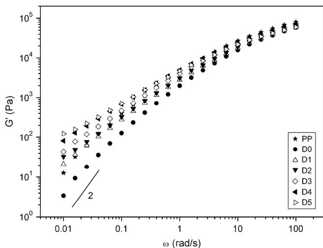
Fig. 5. Storage modulus vs. frequency for the plain PP and modified PPs at 180 °C.
