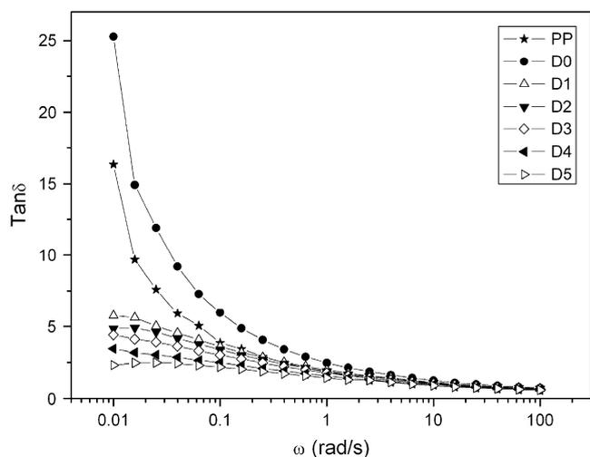
Fig. 6.  $\tan \delta$  vs. angle frequency for the plain PP and modified PPs at 180 °C.
