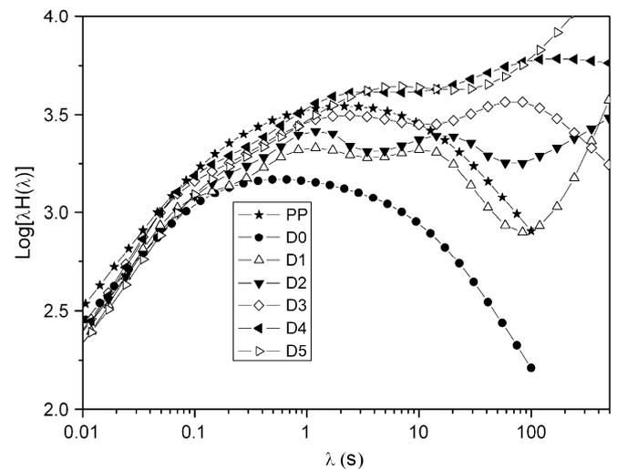
Fig. 9. Weighted relaxation spectrum for the plain PP and modified PPs.
